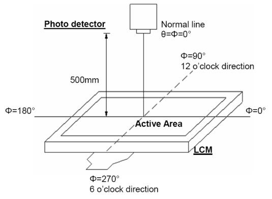
Figure 4.2 Optical measurement system setup
